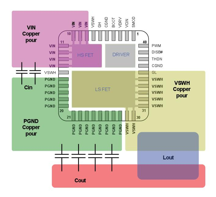
Figure 15. PCB Layout Illustration for Minimizing Current Loops
