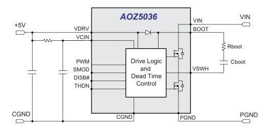
Figure 14. Applying VDRV and Generating BOOT Supply
