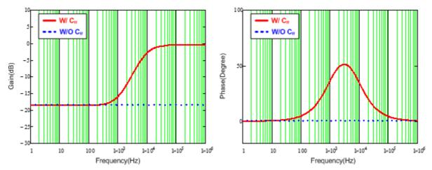
Figure 7. Bode Plot with Different Feedback Loop Conditions
