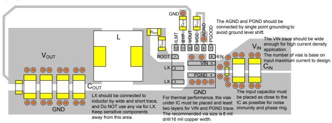
Figure 11. Layout guide of RT6228B.
