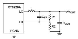
Figure 6. Feedback Loop with feedforward Capacitor.
