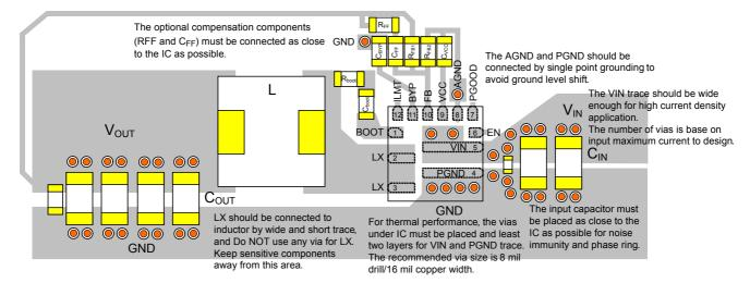
Figure 10. Layout Guide of RT6228A.
