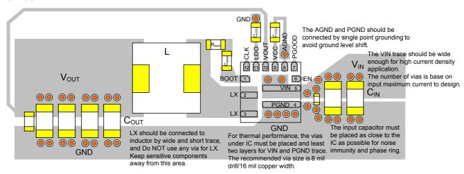
Figure 12. Layout guide of RT6228C.
