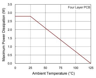
Figure 9. Derating Curve of Maximum Power Dissipation
