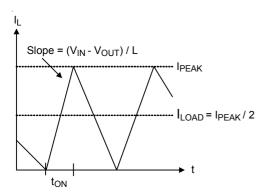
Figure 2. Boundary Condition of CCM/DEM
